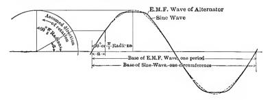
FIG. 41. E. m. f. curve of alternator on time base super-imposed upon sine wave on angle base, showing their similarity.
